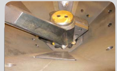
Fixed and rotating rings are used in final crushing stage.
