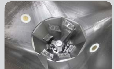
Feed hopper directs material down into the crusher's fixed cast cutters and rotating arm.
