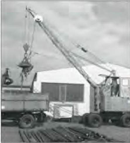
1962: rope-driven S833 with elevated operator cab
