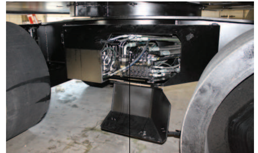
Highly accessible upper and lower main valves make repairs easier.
