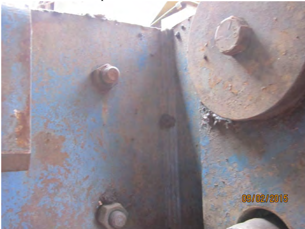
Mid-section pivot clevis welds in excellent condition
