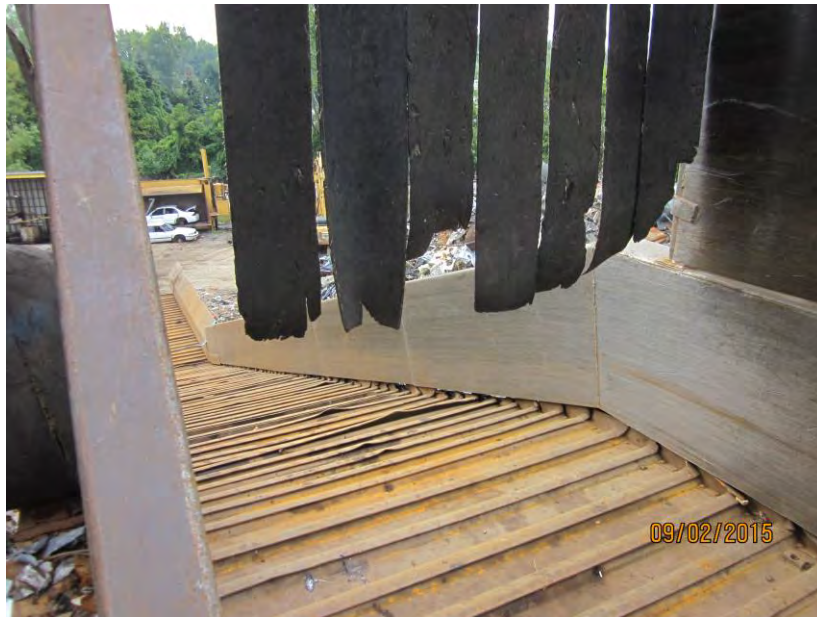
All steel flights in good condition with a few with minor bends
