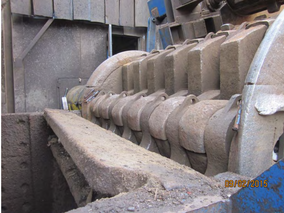
Welded round stock has been added for protecting the cap from hammer wash. They will not last for any length of time as the caps should be replaced
