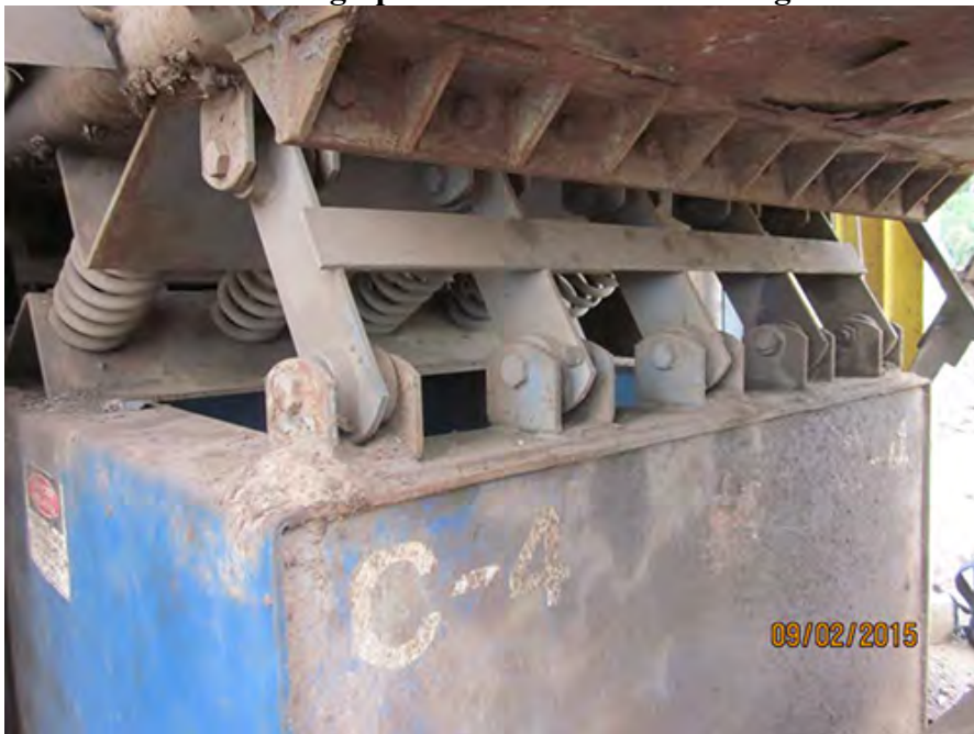
Actuating arms in good condition
