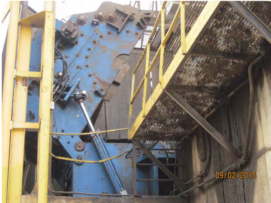
Mid-section and base weldment
