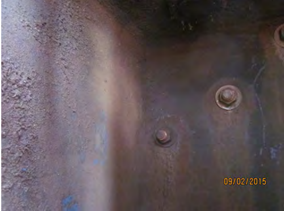
Base section side liner bolts are tight and show no movement
