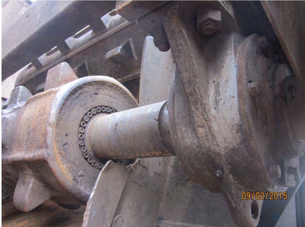
No wire wrap around end of feed roll drum shafts with no evidence of the shafts being gouged from a cutting torch
