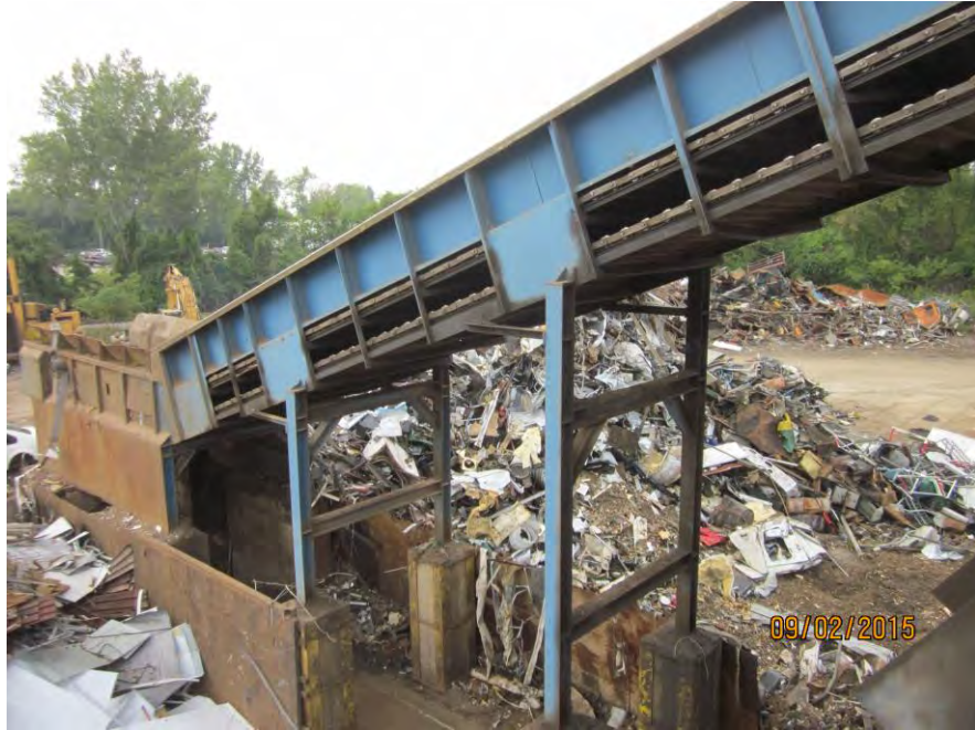
Main Structural Support in good condition. No major material trapped on belt
