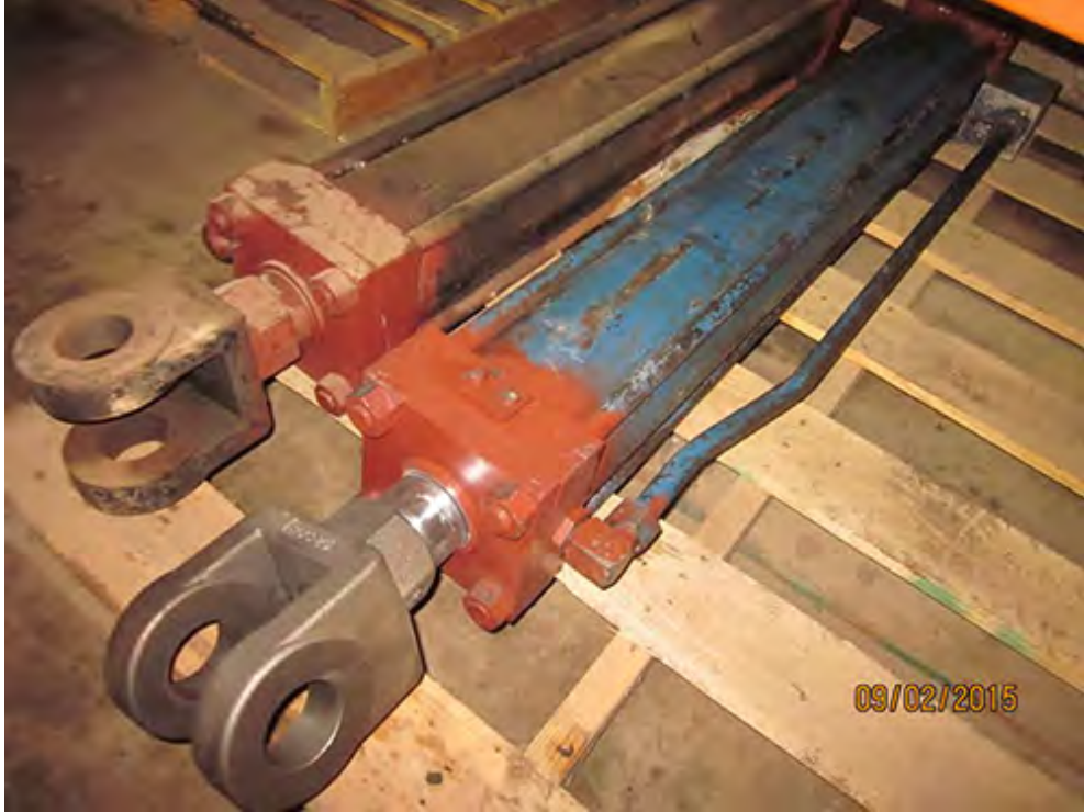
Spare rebuild Mid-section tilt cylinders
