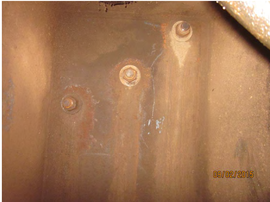
Base section side liner bolts are tight and show no movement
