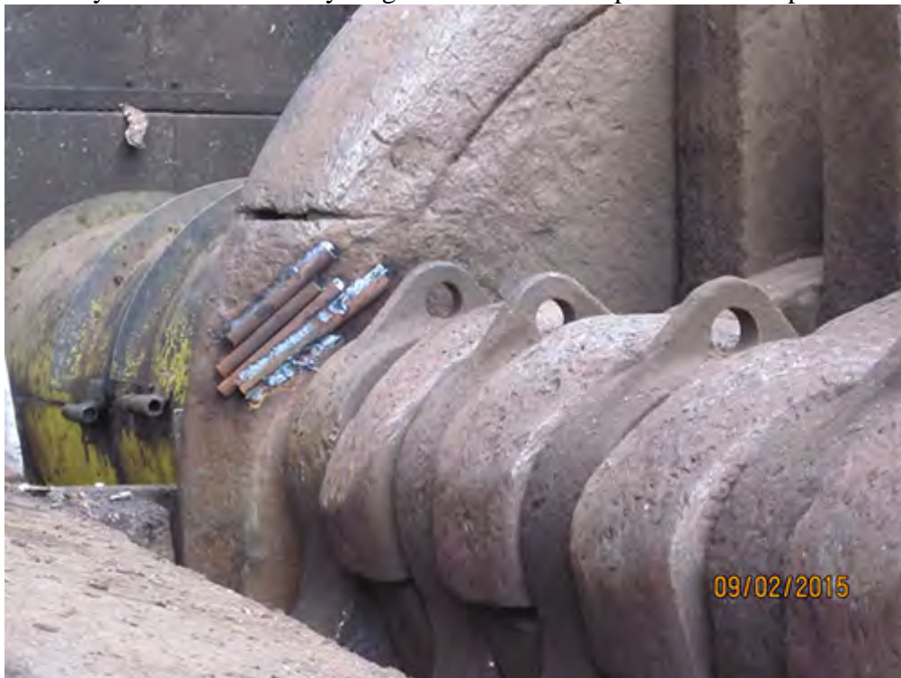
Welded round stock has been added for protecting the cap from hammer wash. They will not last for any length of time as the caps should be replaced
