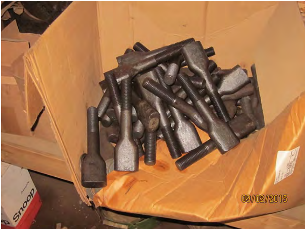
Casting liner bolts
