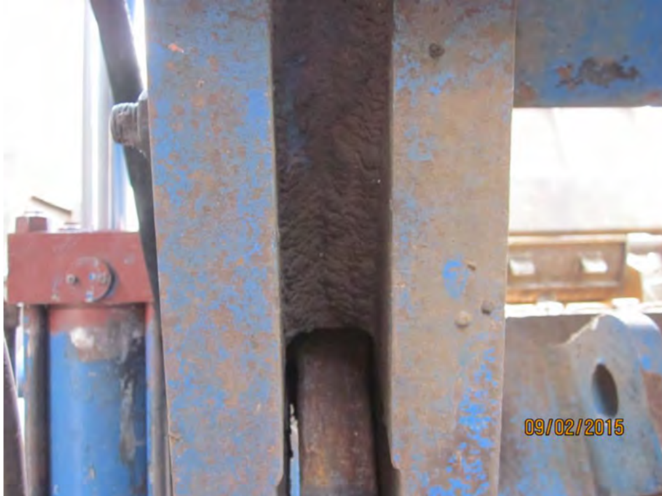
Mid-section pivot clevis welds in excellent condition
