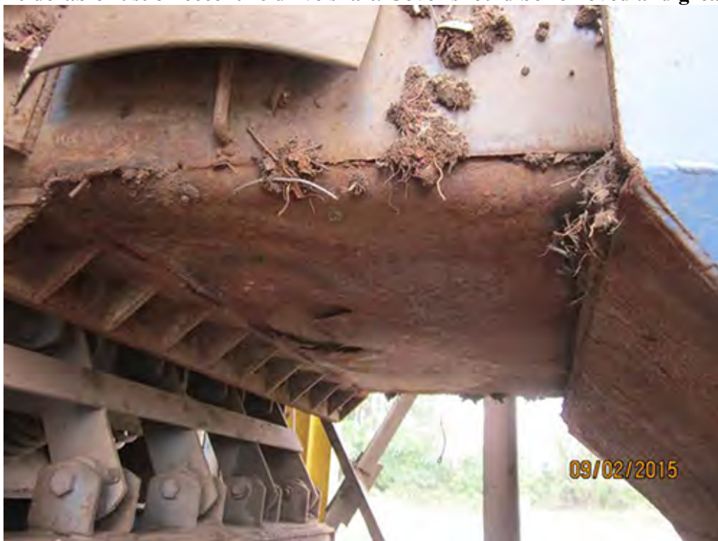
Fisher steel plate should be added to the bottom of the exit chute
