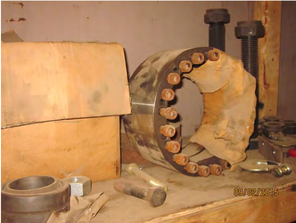
Spare rotor shaft coupling for the 1500 hp motor drive shaft
