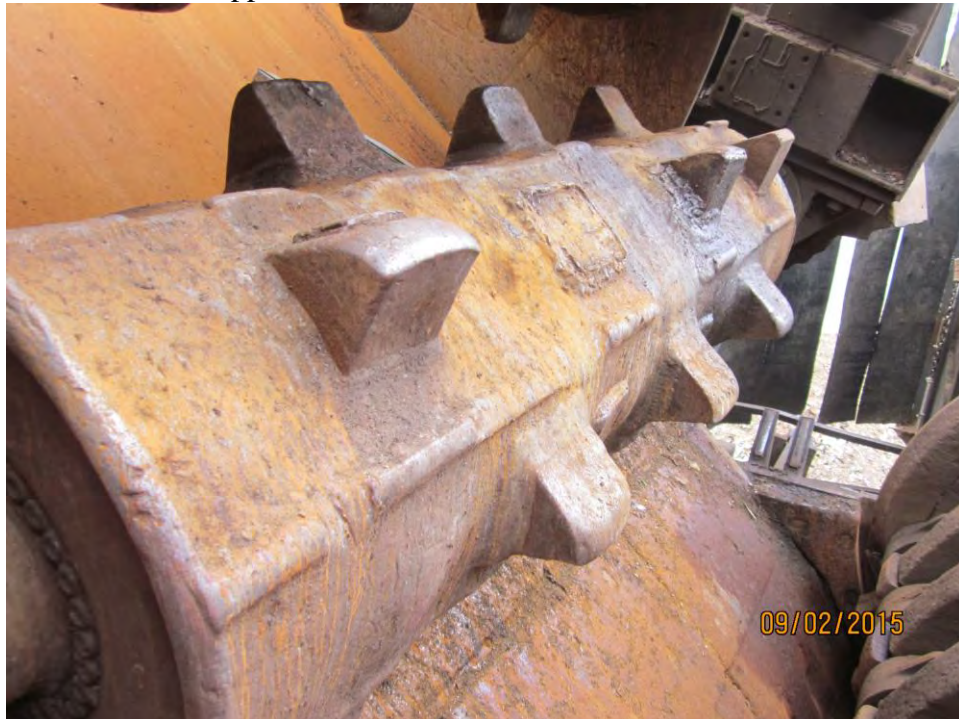
Lower feed roll drum couple teeth missing should be replace. Drum in good condition
