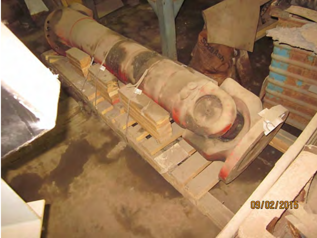
(2) Universal drive shaft for the 2500 hp motor and (1) for the 1500 hp motor not shown
