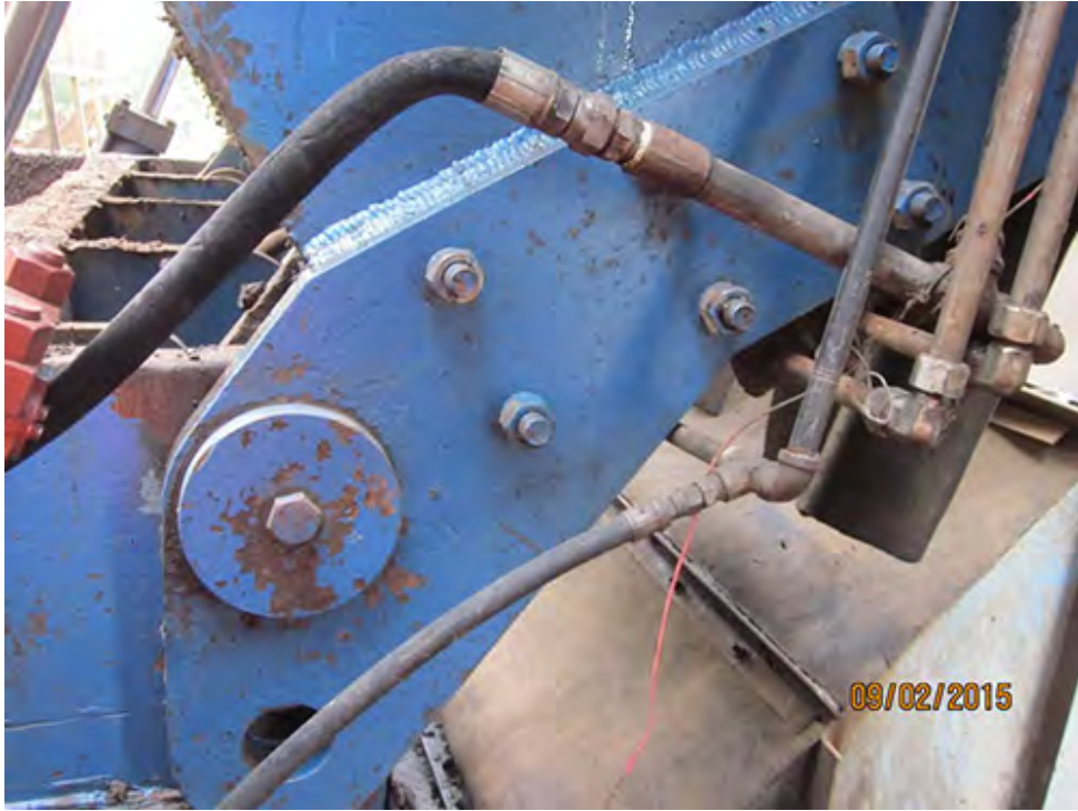
All welds on mid-section pivot arms in good condition
