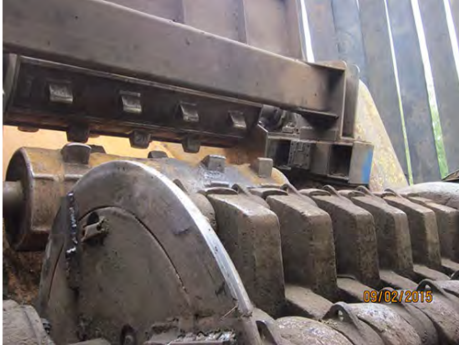
Feed roll frame rectangular cross member torque tube in great shape more robust fabrication added by customer
