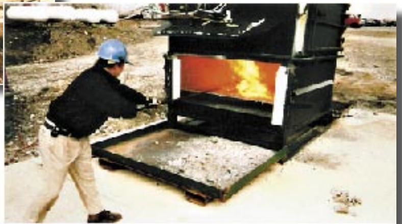
Raking doors (two doors) where slag and iron is removed
