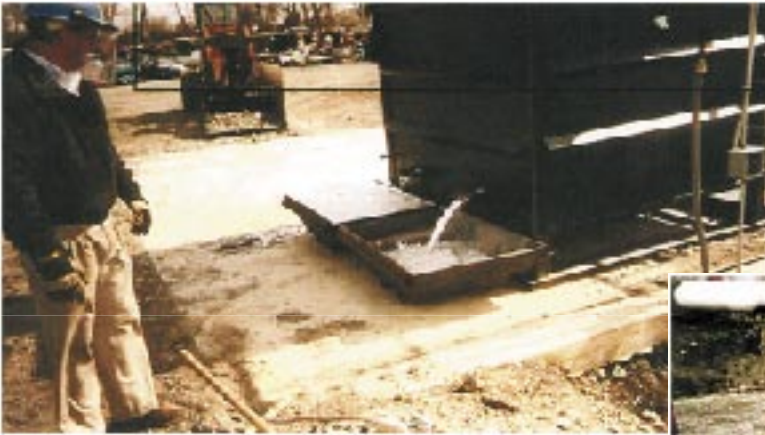
Two 1200lb. sows being poured with the AK8500
