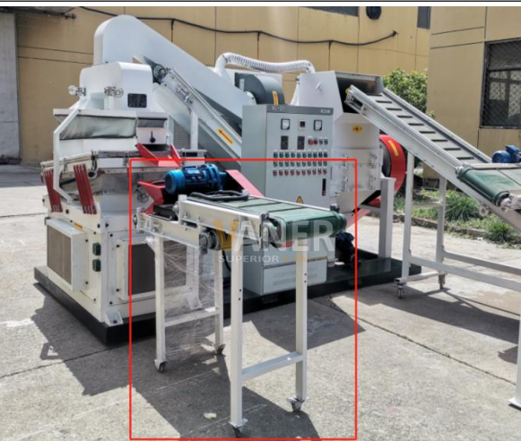
Name: Magnetic separator Power: 1.5kw Quantity: 1 unit Function: Separate other metals from copper granules.
