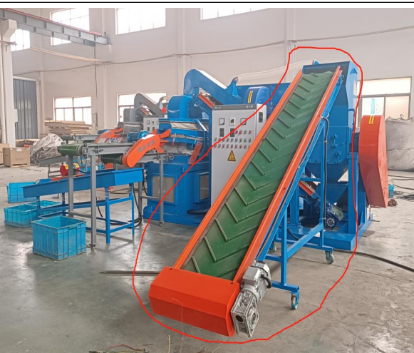
Name: Feeding conveyor Quantity: 1 unit Function: Feeding raw materials into the granulator crusher. * The conveyor not included S30 default device, need buy extra.
