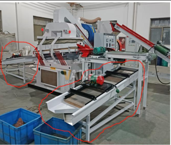
Name: Small vibration tables Power: 0.18kw*2 Quantity: 2 units Function: separate the copper and plastic granules again that out from two outlets .
