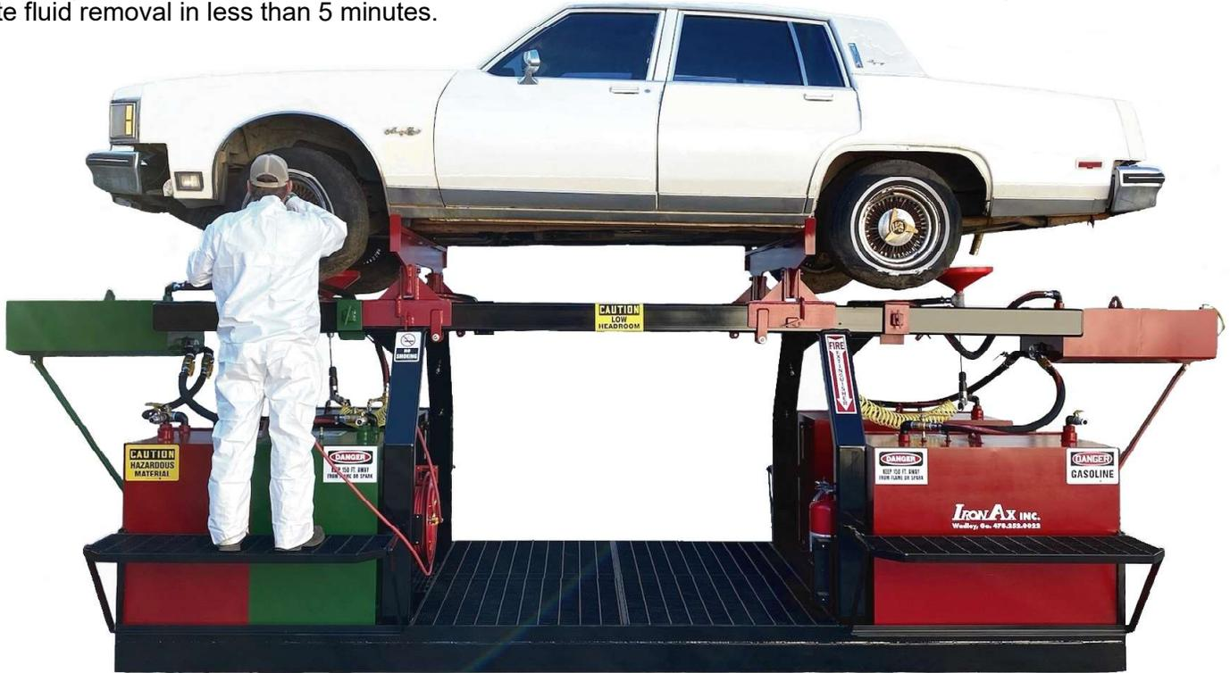
*The Enviro-Rack pictured is equipped with a gasoline separation system, antifreeze separation system, and fold out catwalks.*
